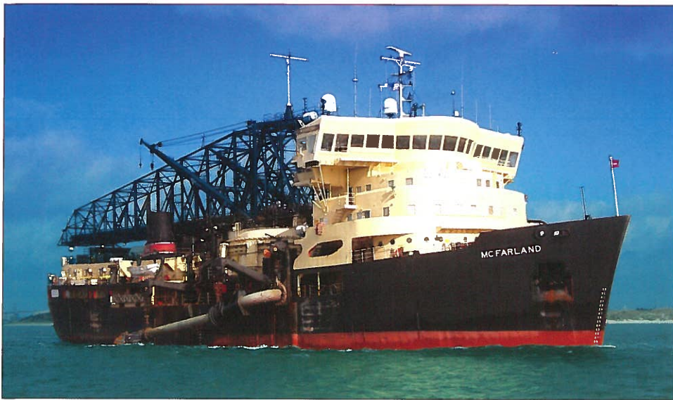
A recent photo of the MCFARLAND, one of four M.E.B.A.-crewed oceangoing hopper dredges owned and operated by the U.S. Army Corps of Engineers. It is the only dredge in the world with triple capability for direct pumpout, bottom discharge and sidelaying or boom discharge.
