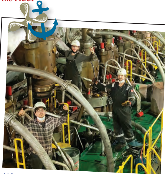
M.E.B.A. officers changing out an exhaust valve on the main engine of the APL vessel PRESIDENT ROOSEVELT. Left to right are 3rd A/E Matthew Farrar, 2nd A/E Kevin Schultz and 1st A/E Trevor Lapham.
